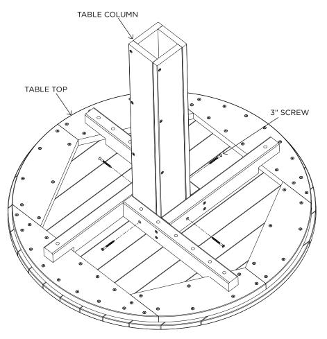
**STEP 3.** Place Table Base on top of the column until the base is flush with the column, use (4) 3" screws to secure the base to the column using pre-drilled holes. Once all screws are fully tightened flip table upright and enjoy!
