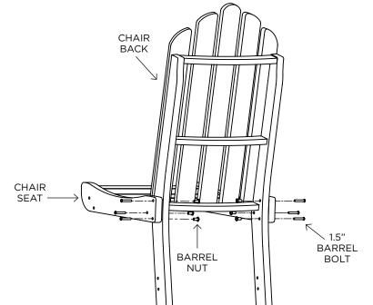
STEP 2. Use (4) 1.5" barrel bolts to attach left and right leg to chair seat. Keep all barrel bolts loose until Step 3.
