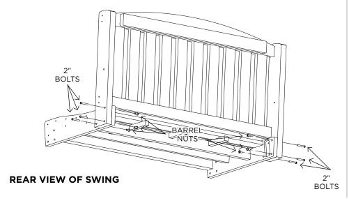
**STEP 3.** Use (6) 2" Bolts, and (6) Barrel Nuts to attach bottom of arms to bench.
