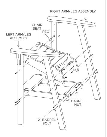
**STEP 3.** Use (2) 1.5" barrel bolts and (2) barrel nuts to attach chair back to right & left arm/leg assembly.
