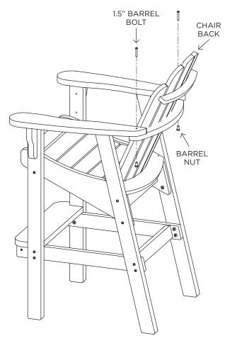
**STEP 4.** Use (2) 2" screws to attach chair back to chair seat. Tighten all bolts once screws are in.
