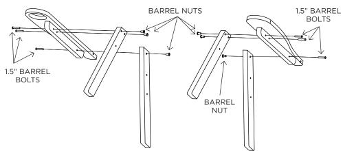
**STEP 2.** Use (2) 2.5" barrel bolts, (6) 1.5" barrel bolts, and (8) barrel nuts to attach arm assemblies & supports to inside of chair frame.
