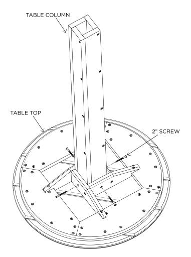
**STEP 3.** Place Table Base on top of the column until the base is flush with the column, use (4) 3" screws to secure the base to the column using pre-drilled holes. Once all screws are fully tightened flip table upright and enjoy!
