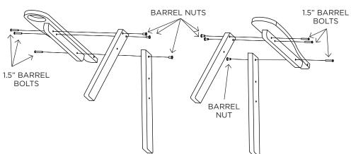
**STEP 2.** Use (2) 2.5" barrel bolts, (6) 1.5" barrel bolts, and (8) barrel nuts to attach arm assemblies & supports to inside of chair frame. **Tighten all bolts for chair; continue to step 3 for rocker.**
