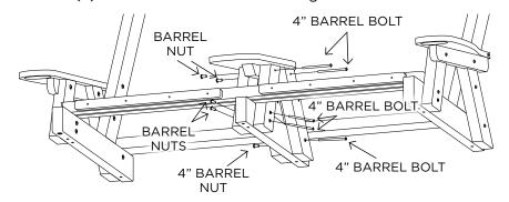
**STEP 5.** Add the center upright and use (2) 4" barrel bolts and (2) barrel nuts to the back table legs. **(Tabletop hidden to see assembly of hardware)**
