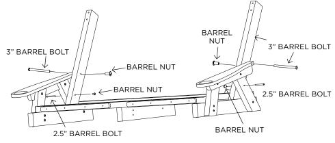
**STEP 4.** Use (2) 4" barrel bolts and (2) barrel nuts to attach front table legs to center beam. Use (1) 4" barrel bolt and (1) barrel nut to attach back table legs to center beam. Then add table top and use (2) 4" barrel bolts and (2) barrel nuts to attach table legs to bottom of table.
