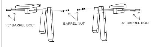
**STEP 2.** Use (6) 2.5" barrel bolts and (6) barrel nuts to attach arm assemblies to outside of frame.
