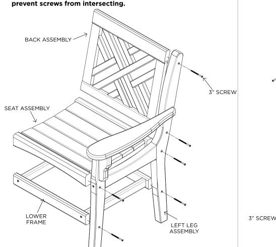
**STEP 2.** Use (6) 3" screws to attach the Right Leg Assembly to the Seat Assembly, Lower Frame, and Back Assembly.
