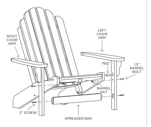
**STEP 3.** Use (2) 1.5" barrel bolts and (2) barrel nuts to attach right & left chair arm to chair back. Tighten all bolts.
