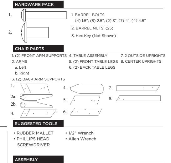
**STEP 1.** Use (4) 1.5" barrel bolts and (4) barrel nuts to attach left arm and right arm to rear and front arm support. **NOTE.** do **not** tighten bolts until Step 5.
