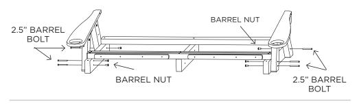
**STEP 3.** Use (2) 2.5" barrel bolts and (2) barrel nuts to attach frame to left and right supports. Use (2) 3" barrel bolts and (2) barrel nuts to attach left and right uprights to arms.
