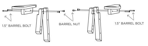
**STEP 2.** Use (6) 2.5" barrel bolts and (6) barrel nuts to attach arm assemblies to outside of frame.
